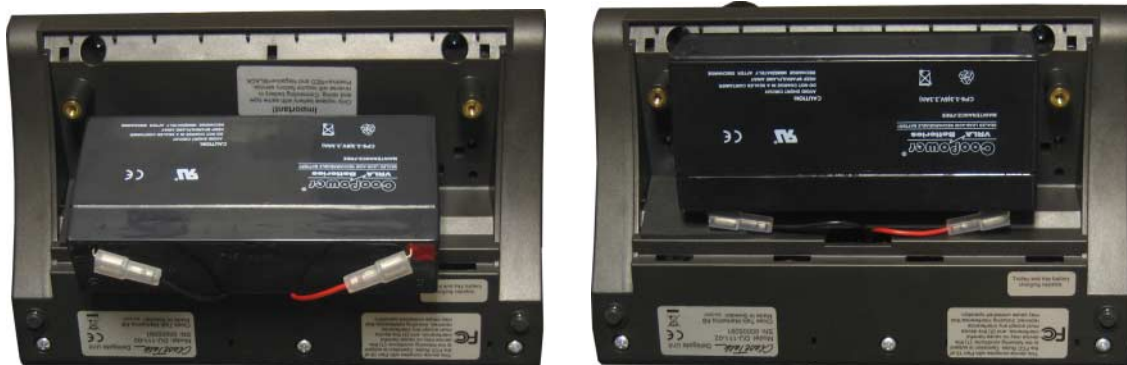
Fig. 30 and 31: Connected battery with correct case position
