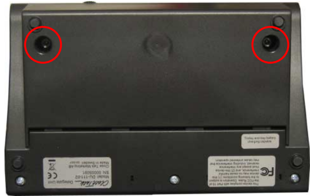
Fig. 3: Battery cover screws
