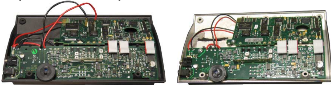
Fig. 23: Top board re-seated, screws returned on metallized case, both cables ready
