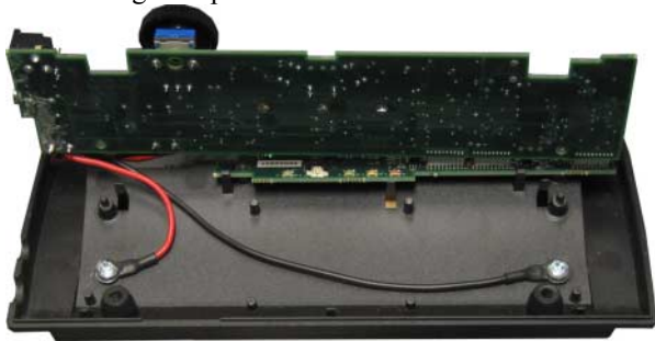
Fig. 22: Both cable ends have been secured
