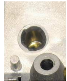
Fig. 20: Metallized case, board lifted and cables inserted
