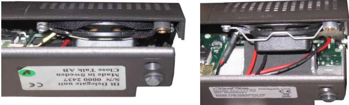
Fig. 28 and 29: Speaker cable arrangement, cable goes under the PC-board
